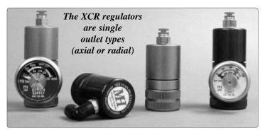
The **XCR** series of regulators are essentially single-outlet. These regulators feature the **SMC** quick-lock system for the 4 mm. and 6 mm. polyurethane tubing. Standard issue with our **XCR** and **EDS** single-place system packages is the 4 mm. radial swivel-elbow regulator. The axial outlet versions are available in CGA-540 & DIN-477 with built-in cylinder pressure gauges.
