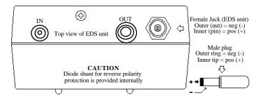
The EDS-EPS (External Power Supply) input jack and plug.
