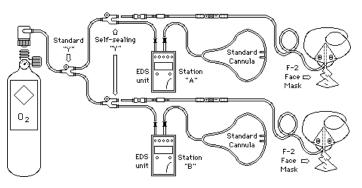
Because many pilots fly with passengers only part of the time, the A-3 flowmeter/regulator and an Oxymizer® cannula can be used for the passenger instead of a second EDS unit. This of course will use more oxygen than each using an EDS, but will prove acceptable as it is less expensive and can be up-graded to an EDS in the future.
