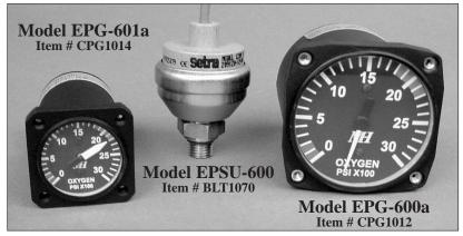
EPG-600a & EPG-601a operate on 10 to 28 VDC with external module. They can be used with any 4-20 ma. (0-3000 psi) current-loop sending unit.
