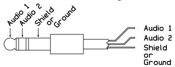
The standard wiring option has one Audio Output wired to the Left Input and the other Audio Output wired to the Right Input.
