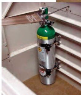
First is the most basic application using the oxygen outlet kits with self sealing CPC style fittings. We have a number of cylinder hold-down kits for aluminum and composite-fiber-wound cylinders.
