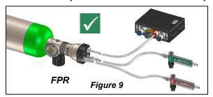
Use the XCP-to-EDS Supply Adapter tubing (00EDS-1070-00) that came with your EDS unit to connect the EDS to the FPR. MH3 and MH4 constant-flow devices connect directly to the CPC connector ports on the FPR regulator.
