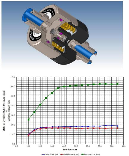
Our step-down pressure regulators have a virtually flat outlet pressure regulation curve for both lock-up (static) and flowing (dynamic) with inlet pressure from 20 to 85 psig. Flows of 40 to 60 liters/minute are measured through a controlled pneumatic resistance with inlet pressures of 20 to 85 psig. Target flows are  $60 \pm 5$  liters/minute throughout the inlet pressure range of 35 to 85 psig.
