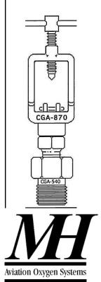
The purpose of this device is intended to allow CGA-540 equipment to be used with CGA-870 (USA Medical) valve equipped cylinders at pressures up to 3,000 psig. (207 bar)
