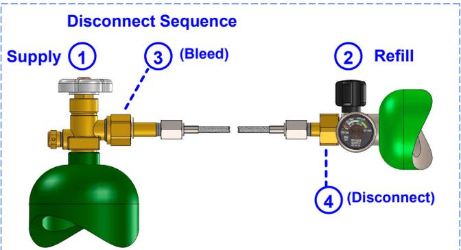
8. Repeat the entire process to fill additional cylinders. If regularly filling more than one cylinder at a time, consider using a TR-75, TR-95 or TR-105 Transfiller. These models incorporate a bleed valve and are therefore more convenient and efficient for multiple refills as they do not require the Supply cylinder fitting to be loosened/bled for each successive Refill cylinder. Also, less Oxygen is wasted, as the entire transfiller does not need to be completely bled between cylinders.
