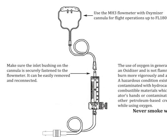
The use of oxygen in general aviation is quite safe. Oxygen is an Oxidizer and is not flammable. Materials which burn will burn more vigorously and at higher temperature in oxygen. A hazardous condition exists if oxygen equipment becomes contaminated with hydrocarbons such as oil, grease or other combustible materials which may include oil from the operator's hands or contaminated tools. Do not use Vaseline or other petroleum-based creams and lotions on your face while using oxygen.
