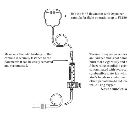
The use of oxygen in general aviation is quite safe. Oxygen is an Oxidizer and is not flammable. Materials which burn will burn more vigorously and at higher temperature in oxygen. A hazardous condition exists if oxygen equipment becomes contaminated with hydrocarbons such as oil, grease or other combustible materials which may include oil from the operator's hands or contaminated tools. Do not use Vaseline or other petroleum-based creams and lotions on your face while using oxygen.
