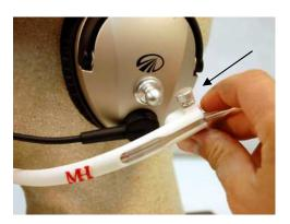
2: Cut out the joint fitting in the tubing located about two inches down from the arm mount.
