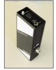
The Flowtimer by Spiegelberg in Hamburg adjusts electronically to the pilot's breathing rhythm. The pilot has to select the oxygen pulse length to suit the specific altitude.
