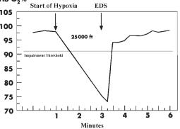
At high altitudes loss of oxyen supply is immediately critical. EDS provides rapid relief.
