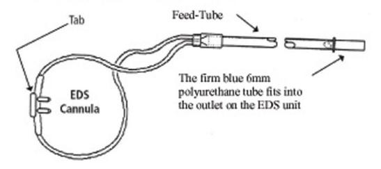
Your nasal cannula should be inspected before each flight and replaced if cracked, plugged, or excessively soiled.
