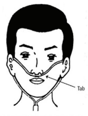
The cannula must be worn with the tab pointing down towards the upper lip.
