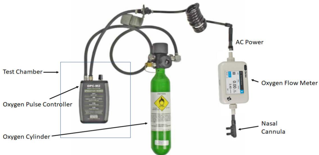
Figure 2-1: General Electromagnetic Test Configuration
