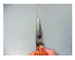
5: The cut end of the vinyl tubing will now have to be stretched to fit over the new adapter sleeve. This can be done by immersing the cut tube end in HOT water, inserting clean needle nose pliers and pulling the handles apart.
