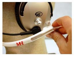
2: Slide the vinyl retaining ring off towards the cannula tip and set aside. Note the position of the arm for easier repositioning.
