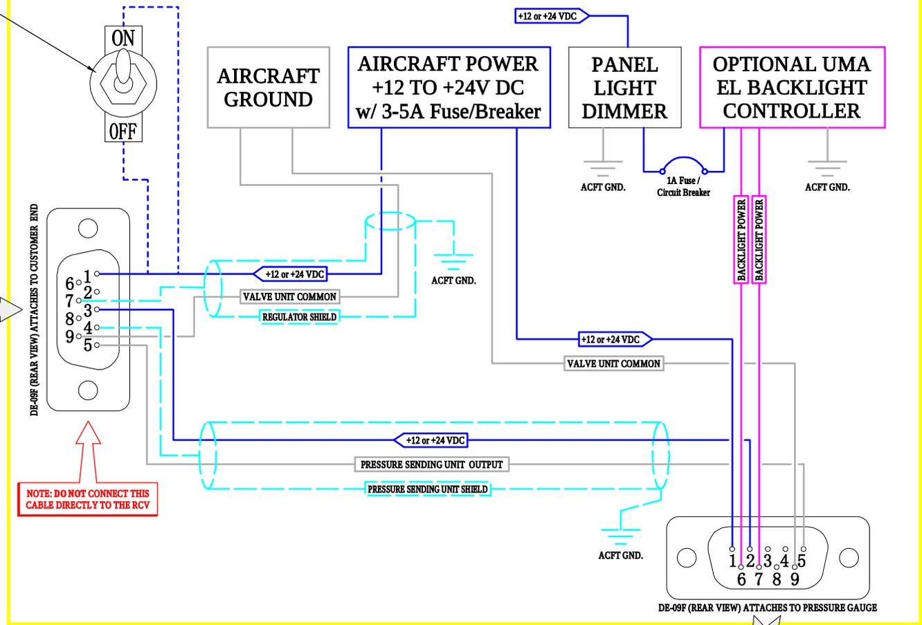
NOTE: DO NOT CONNECT THIS CABLE DIRECTLY TO THE RCV
