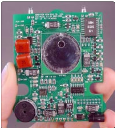
The EDS-D1 internal PCB module showing analog & digital state-of-the-art micro-electronic components.
