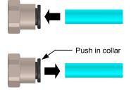
When removing tubing, <u>DO NOT</u> pull on the tubing without pushing in the collar, as this will likely damage the connector. A video on the MH website provides more information about tubing connection.
