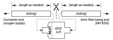
A typical arrangement is to leave a short piece of tubing on the *connector* end so that the EDS-ILR is positioned close to the built-in oxygen outlet as illustrated in the photo at right. In this case the light-weight EDS-ILR simply hangs from the overhead oxygen port. The tubing may also be cut longer to allow you to position the EDS-ILR elsewhere should you prefer.
