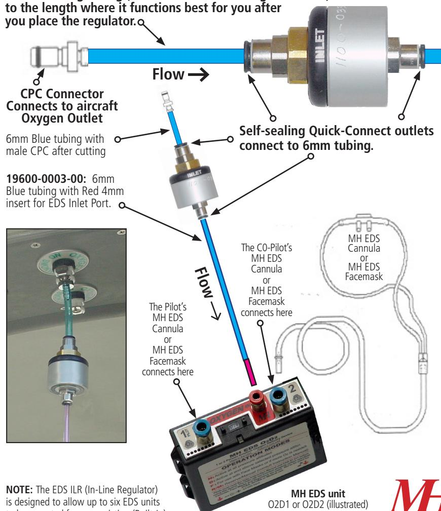
**NOTE:** The EDS ILR (In-Line Regulator) is designed to allow up to six EDS units to be operated from an existing (Built-In) oxygen system where the pressure is 20 to 90 psig.
