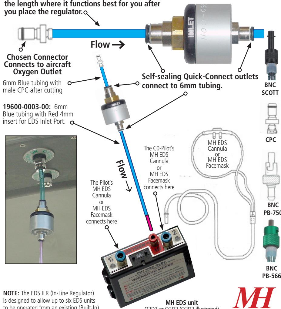
**NOTE:** The EDS ILR (In-Line Regulator) is designed to allow up to six EDS units to be operated from an existing (Built-In) oxygen system where the pressure is 20 to 90 psig.
