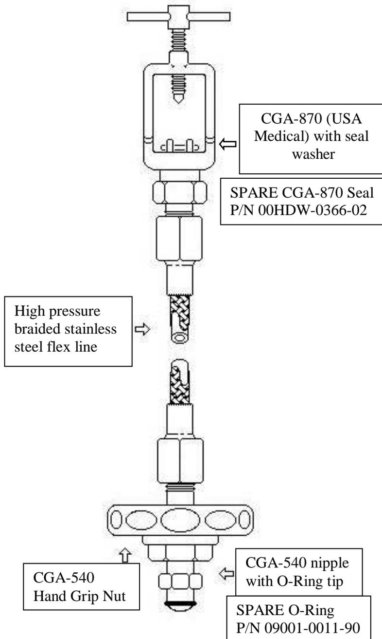
1. Make sure the cylinder fittings are proper CGA Type and are in good shape and completely free of any oil, grease or dirt.
