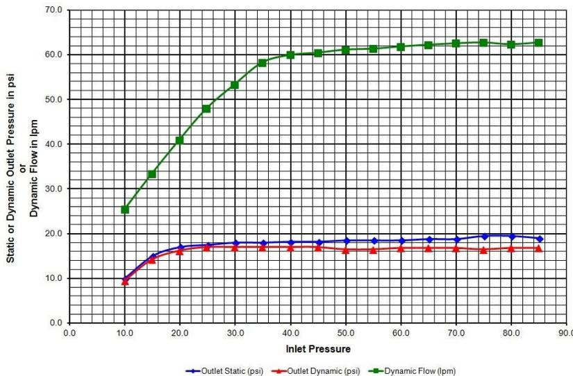
Our step-down pressure regulators have a virtually flat outlet pressure regulation curve for both lock-up (static) and flowing (dynamic) with inlet pressure from 20 to 85 psig. Flows of 40 to 60 liters/minute are measured through a controlled pneumatic resistance with inlet pressures of 20 to 85 psig. Target flows are  $60 \pm 5$  liters/minute throughout the inlet pressure range of 35 to 85 psig.
