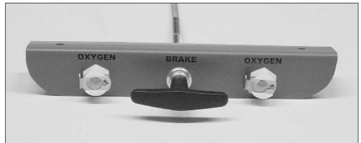
Oxygen outlet fittings mounted in a panel that will be placed just below the center console
