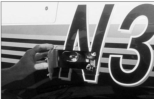
The remote-fill station with gauge mounted next to the external electrical connector behind a flush-fitting access door
