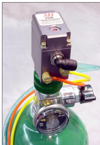
The PCR regulator directly connects (by hand) to the service/refill port of any oxygen cylinder with the standard CGA-540 (USA) or optionally DIN-477 (Euro) valve allowing the cylinder to be easily removed for refilling or service. An auxiliary port on the rear side of the regulator body (not shown) is provided for an optional remote oxygen fill station and pressure gauge.
