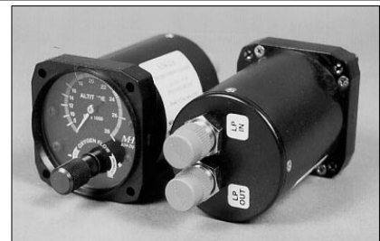
The PCR regulator directly connects (by hand) to the service/refill port of any oxygen cylinder with the standard CGA-540 (USA) or optionally DIN-477 (Euro) valve allowing the cylinder to be easily removed for refilling or service. An auxiliary port on the rear side of the regulator body (not shown) is provided for an optional remote oxygen fill station and pressure gauge.
