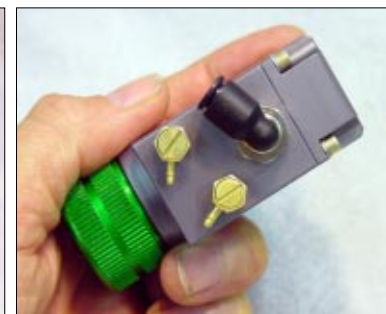
The PCR regulator directly connects (by hand) to the service/refill port of any oxygen cylinder with the standard CGA-540 (USA) or optionally DIN-477 (Euro) valve allowing the cylinder to be easily removed for refilling or service. An auxiliary port on the rear side of the regulator body (not shown) is provided for an optional remote oxygen fill station and pressure gauge.
