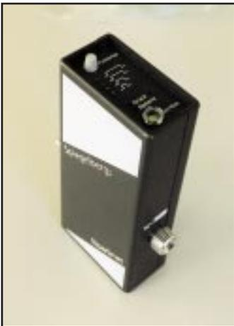
The Flowtimer by Spiegelberg in Hamburg adjusts electronically to the pilot's breathing rhythm. The pilot has to select the oxygen pulse length to suit the specific altitude.
